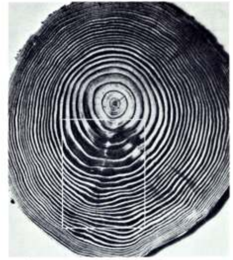
Compression wood showing unusual ring pattern and cracks across the rings.
